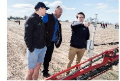
Technology coming to agriculture. Here is a new machine vision + artificial intelligence system which is able identify and spray green weeds in a green crop. This means less pesticide in the environment, better weed control and potentially higher crop yields.
