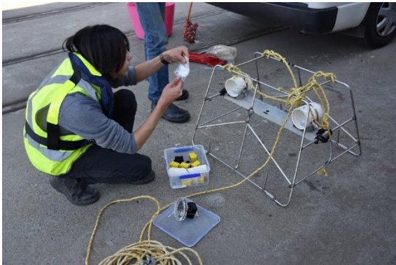
UWA Field Techniques students collaborate with Southern Ports Albany staff to prepare the Stereo Baited Remote Underwater Video Systems (BRUV) for deployment at Albany Port.
